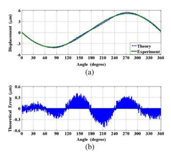
Fig. 6 Experimental results of axial slip measurement: **a** a full rotation, **b** theoretical error
