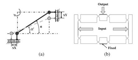
Fig. 9 Flexure hinge mechanism: a dimensional parameters, b FEA results
