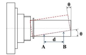
Fig. 3 Measurement of spindle tilt angle
