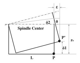
Fig. 4 Spindle tilt-generated axial slip
