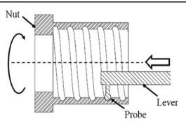
Fig. 1 Measurement principle of the ballscrew nut
