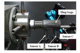
Fig. 5 Setup of tilt and axial slip measurement
