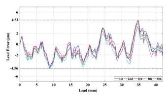
Fig. 14 Measured cumulative-lead errors of a ballscrew nut
