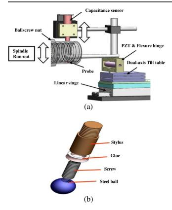
Fig. 7 Schematic of run-out compensation, **a** the measurement system and **b** the probe assembly
